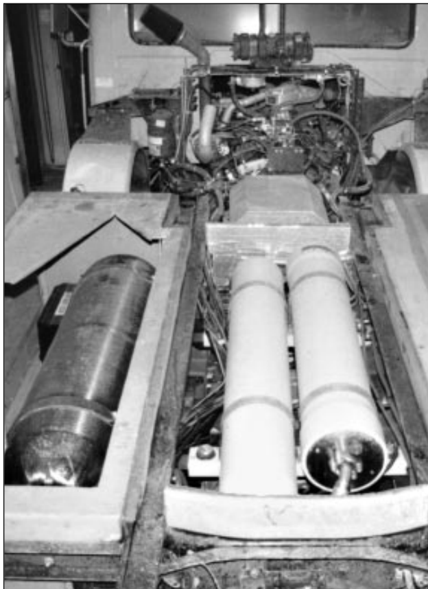
Assembly of refuse collection vehicle
